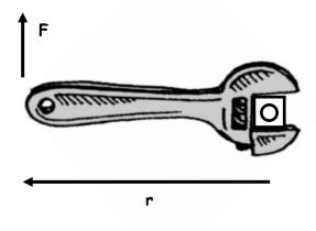
B. Torque = lever arm (r) x perpendicular force (F).
