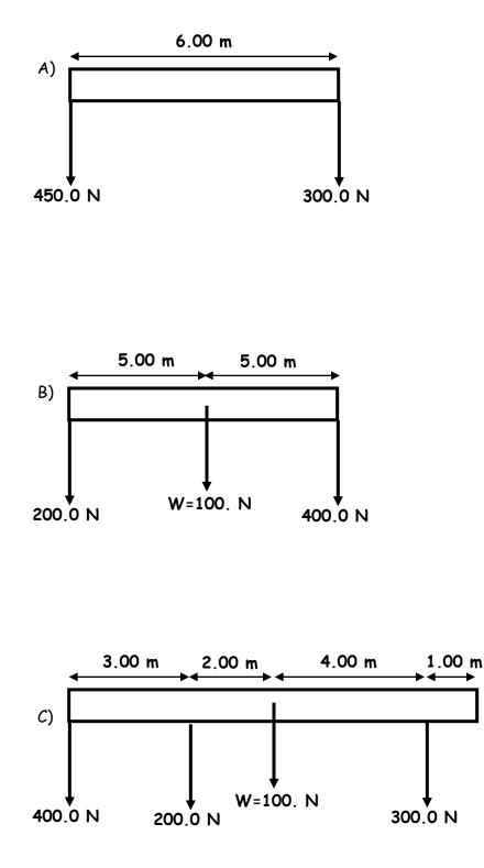
**III**. Find the force, F, needed to balance the bar. In cases A) and C), assume the bars have negligible mass. In case B), the location of the center of mass is again designated by the downward arrow and the W.
