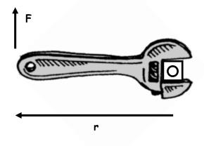
B. Torque = lever arm (r) x perpendicular force (F).
