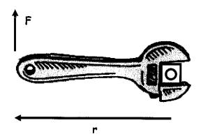
B. Torque = lever arm (r) x perpendicular force (F).
