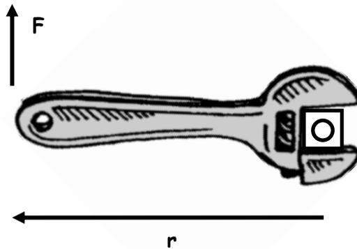
B. Torque = lever arm ( $r$ )  $\times$  perpendicular force ( $F$ ).
