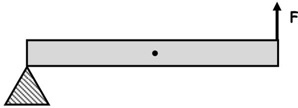
5. Find the force needed to hold the same beam level with the addition of a hanging weight.
