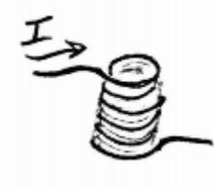
12. Relative to an observer looking downward through the solenoid, which way is current traveling?
