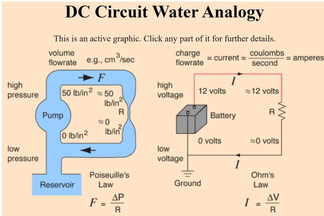
3. In the water circuit, above, what makes the water move?
